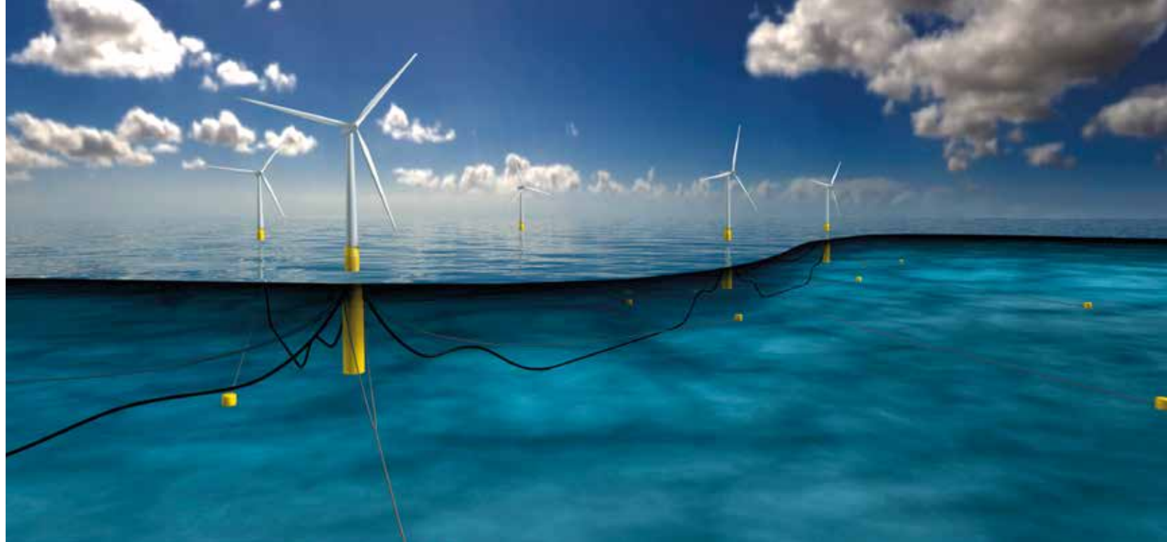
In the Norwegian Hywind concept, wind turbines are placed on a floating buoy with ballast at 80 metres' depth, moored to the seabed.
