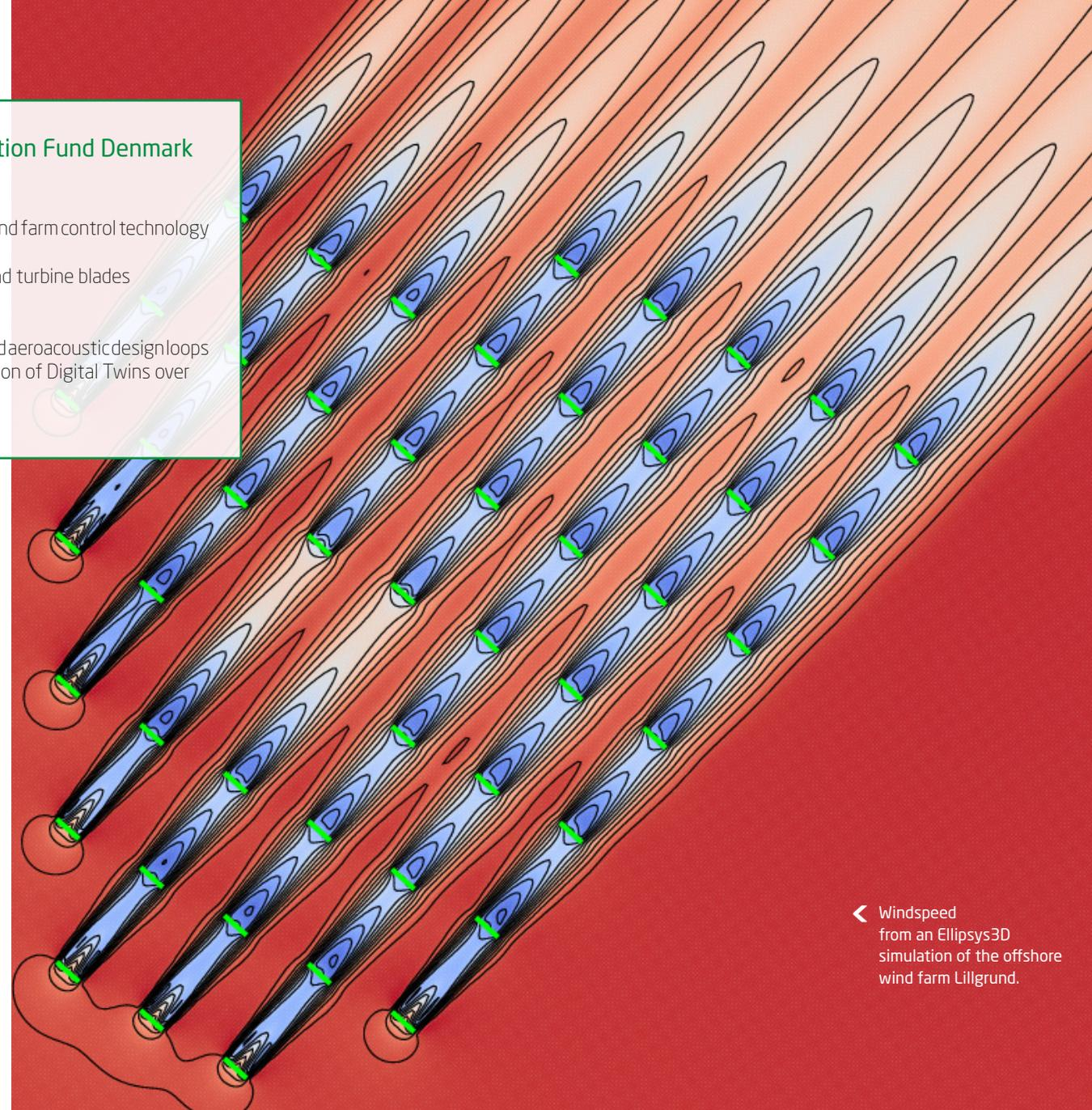
◀ Windspeed from an Ellipsys3D simulation of the offshore wind farm Lillgrund.
